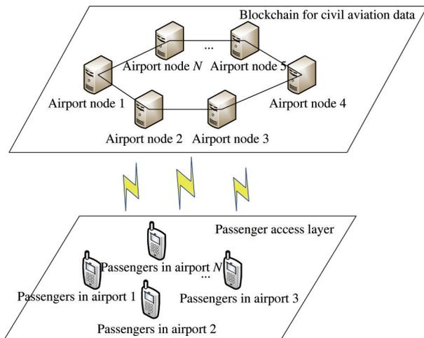
**Fig. 1** System architecture of the blockchain for civil aviation business data
