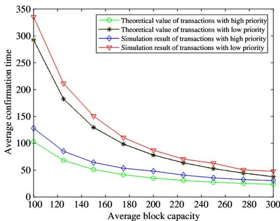
Fig. 5 Impact of average block size  $\lambda_B$  on average confirmation time of transactions with different priority
