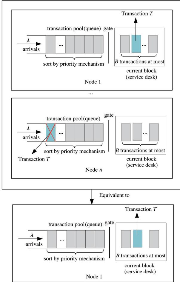
**Fig. 3** A batch-service M/G/1 queuing system with threshold  $B$
