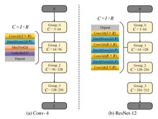
**Fig. 3** Detailed network structure of feature extractors  $v_i^0 = f_\theta(x_i)$
