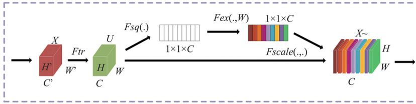
Fig. 3 Squeeze-and-excitation mechanism
