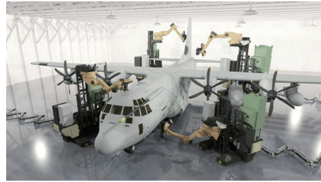
(b) Carnegie Mellon University military aircraft surface coating laser stripping system
