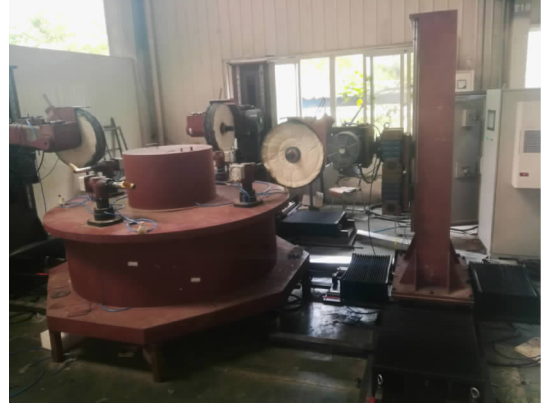
Fig. 15 The multi-station rotary polishing robot at factory
