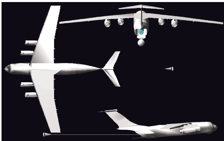
Fig. 2 The three dimensional solid model of internally carried air-launchedLaunch vehicle
