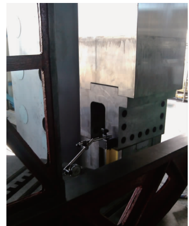
Fig. 7 The test device of vertical hydrostatic guide rail
