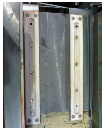
Fig. 2 The oil recess structure
