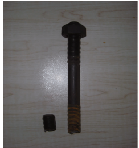
Fig. 12 Cracked M20 bolt
