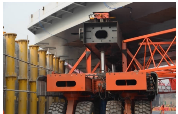
(b) Double vehicles with bridge driving in parallel on the cross-slope Fig. 12 The scene of 1000t BTLV bridge transporting
