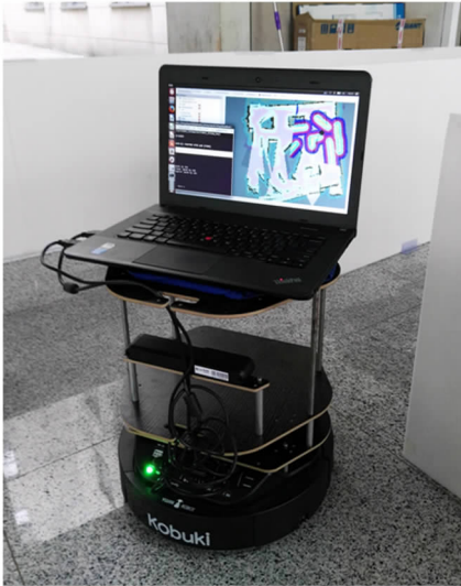
Fig. 10 The Turtlebot2 robot equipped with a Kinect
