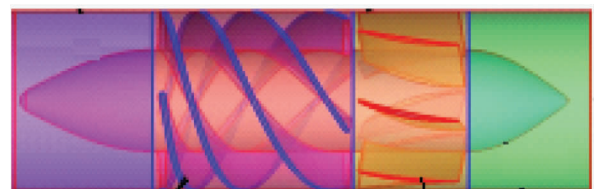
Fig. 5 Computational domain of the pump
