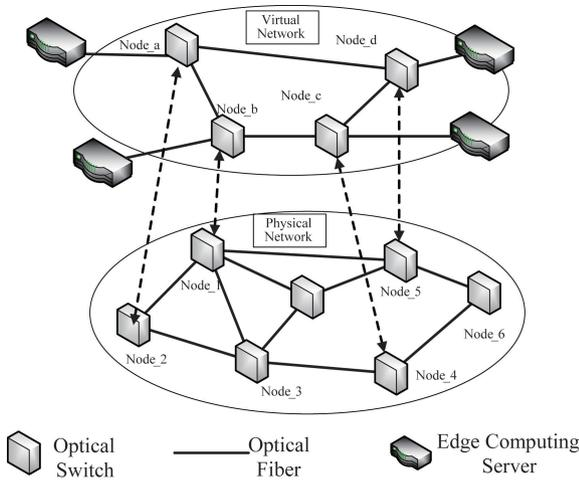
**Fig. 1** Typical architecture of edge computing virtual network
